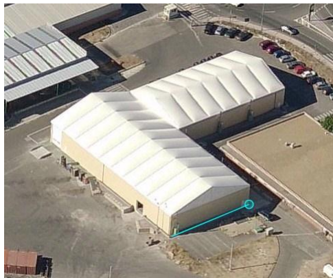
Figure 55: Measuring façade area: Define baseline first...
